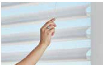
UltraGlide® Operating Wand Ergonomically designed, this retractable wand system controls vane adjustment and the raising of shades by pulling the wand straight down with short strokes. To lower the shading, pull the wand out toward the room and with one click, the shading will release.
